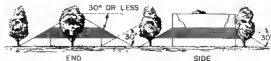
Figure 62. On small buildings where the slope of the roof is 30 degrees or less, the netting runs completely around the building, starting at the eaves and extending only far enough beyond the eaves to mask the ground line of the building when viewed from an angle 30 degrees above ground level.
